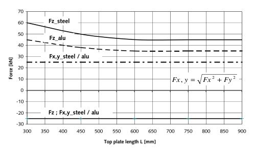
Fig. 5: Measuring ranges
