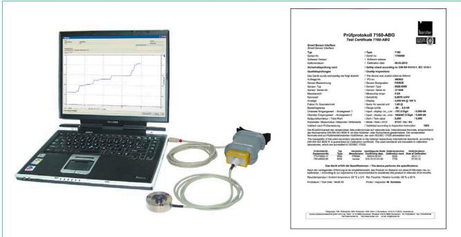
Smart Sensor Interface model 7160 is powered via the USB port of the connected PC which also generates the supply voltage of 4.5 V for the load cell. Via Plug & Measure connection, the data of the connected load cell can be detected. Continuous measurements can be recorded automatically with the Configuration and Data Logging Software DigiCal, so that without considerable effort a test sample can be evaluated for compliance with the technical data.
