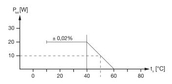
The max. load capacity with different ambient temperature as a function of the warm-up error can be taken from the load reduction curve. Example: Ambient temperature: max. 50°C; accepted  $\triangle$  R by temperature influence: max. 0.02 %; max. permissible load: 10 W.
