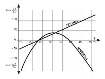
The graph above shows the theoretical relationship between the temperature coefficients and the change in resistance as a function of the temperature, i.e. the ideal characteristics for MANGANIN<sup>®</sup> and ZERANIN<sup>®</sup>. We constantly strive to manufacture resistors with similar characteristics through the careful selection and appropriate processing of the MANGANIN<sup>®</sup> or ZERANIN<sup>®</sup>.
