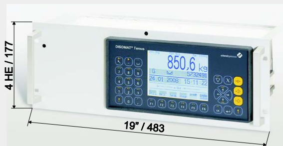
19" VNG 20450 sub-rack with built-in VEG 20450 terminal Depth 195 mm + 25 mm for service cable Protection class: front IP 54 otherwise IP 20 Weight: 7.5 kg
