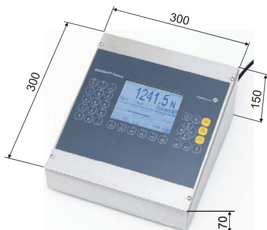
Stainless steel VKG 20450 housing Table-top mounting Protection class: IP 65 (NEMA 4x) Weight: 5 kg The VKG 20450 can also be mounted on the wall with the attached holder. (cable outlets below)
