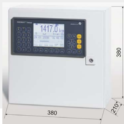
VFG 20450 crane/field housing with built-in VEG 20450 terminal, Sheet steel, Protection class: IP 54, Weight 11 kg * 230mm incl. the front frame
